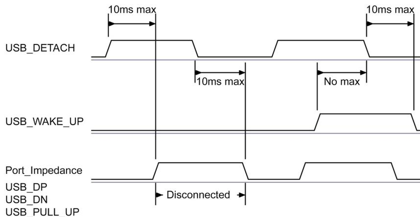
Figure 11.17: USB\_DETACH and USB\_WAKE\_UP Signal
