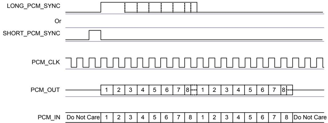
Figure 11.24: Multi-slot Operation with Two Slots and 8-bit Companded Samples
