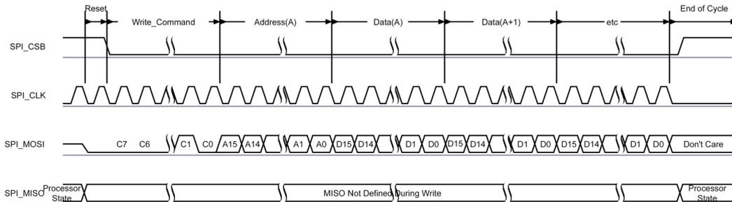
Figure 11.18: Write Operation
