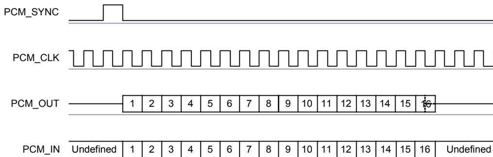
**Figure 11.23: Short Frame Sync (Shown with 16-bit Sample)**
