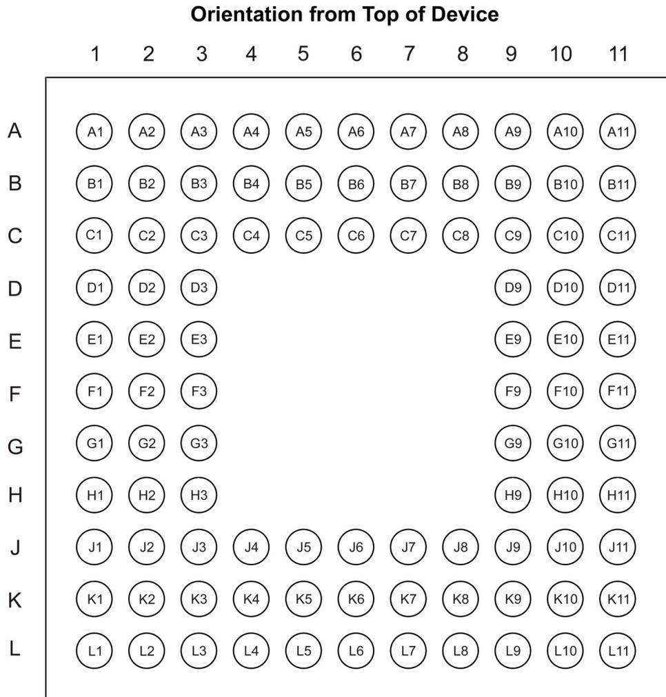
Figure 3.1: BlueCore4-External 8 x 8mm Device Pinout (BC417143B-IQN-E4)
