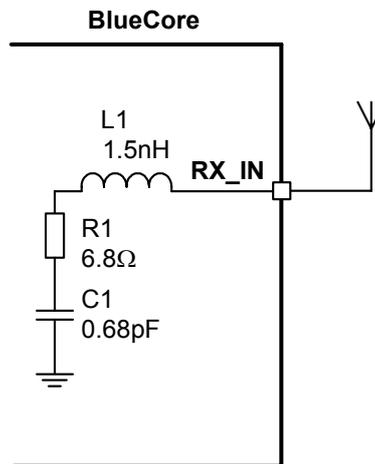
Figure 11.2: Circuit RX\_IN
