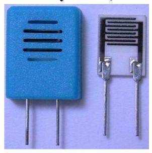
**1.** HR202 is a new kind of humidity-sensitive resistor made from organic macromolecule materials, it can be used in occasions like: hospitals, storage, workshop, textile industry, tobaccos, pharmaceutical field, meteorology, etc.
